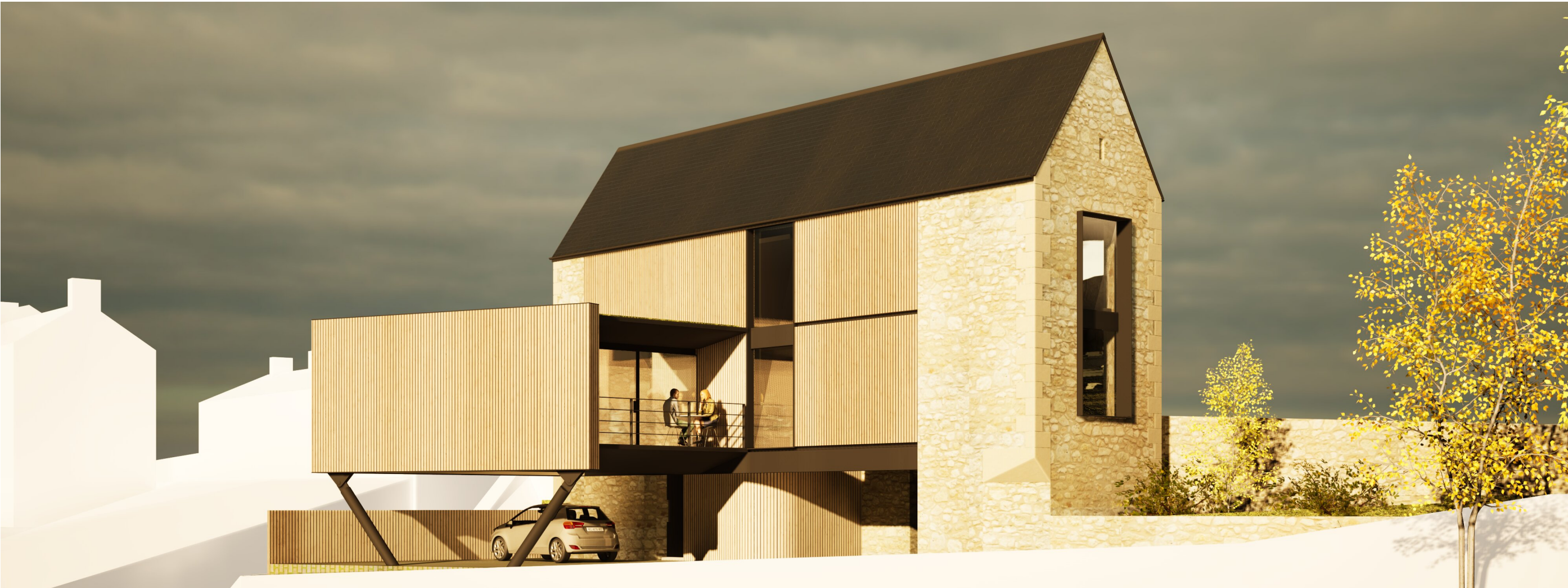
Fig 10. Living accommodation and amenity terrace back onto the railway line and are shielded by a wrap around roof / wall. Openings in the adjacent wall are acoustically attenuated serving non-habitable accommodation only.
